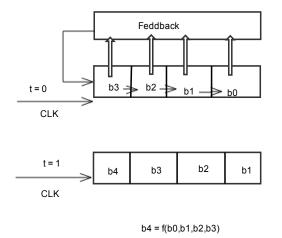
Figure 1: Digaram of a shift register with feedback
